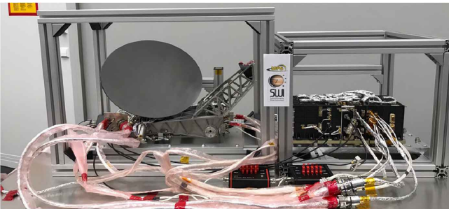
Fig. 17. SWI instrument. The offset Cassegrain system and receiver unit is on the left. The electronic unit is on the right
