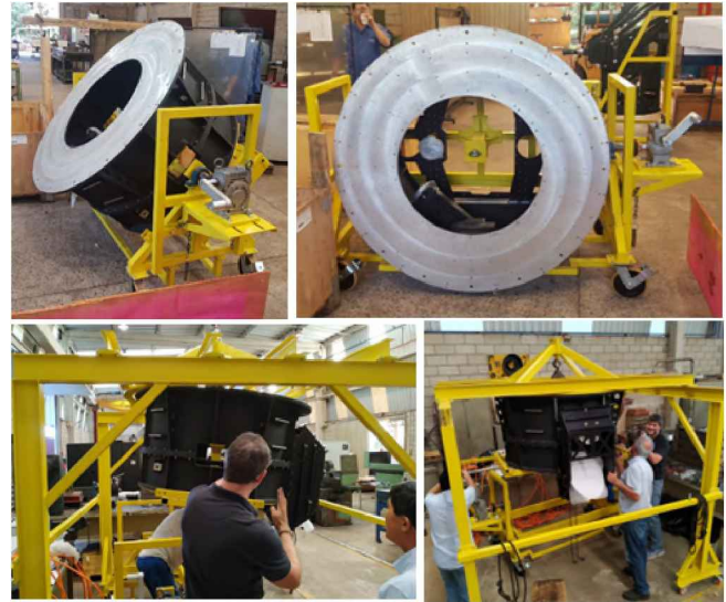
Fig. 7. The handling and installation of the NACOS's CASS structure in the Cassegrain Cabin emulator fixture.
