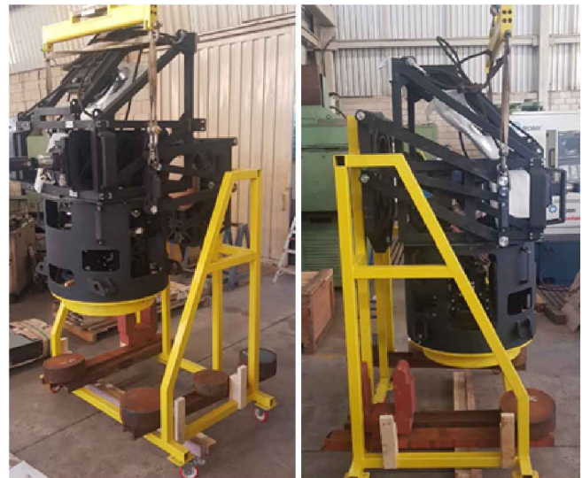
Fig. 8. Testing of the NACOS's NASS structure fixed in the Nasmyth Cabin interface emulator fixture.
