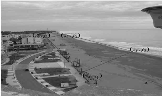
Figure 2: Control Points ((x_1, y_1), (x_2, y_2), (x_3, y_3), (x_4, y_4)) whose geographic coordinates were obtained with a Global Positioning System and are related with the pixels coordinates in the image.
