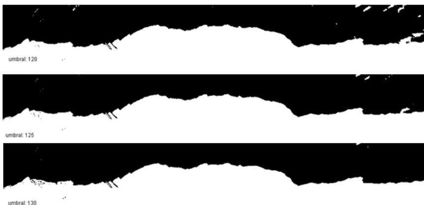
Figure 7: Images binarized with different threshold values. Empirically, the middle one performs best in the further processing steps.
