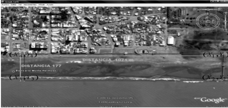
Figure 3: GPS-established control points taken in the image. These geographic coordinates determine the parameter of the projection matrix.
