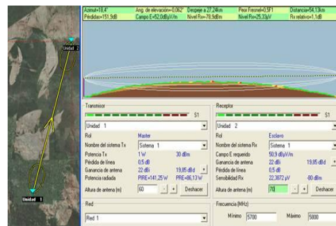
Figure 8: Results from elevating antenna height at frequency 5.7 GHz
