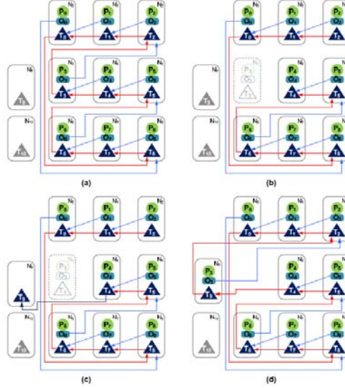
Fig. 2. Phases in the fault recuperation process of node 3, using 2 spare nodes.
