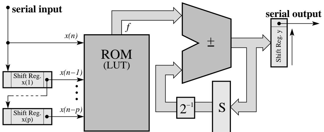
Figure 3: FIR-Filter Architecture.
