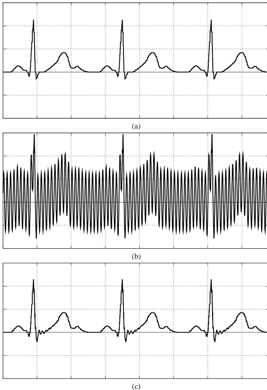
Figure 5: Removing mains-frequency interference from an electrocardiogram.
