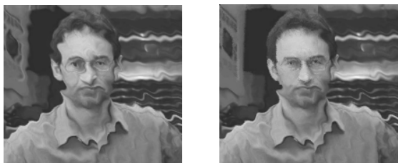
Figura 11c. Block Matching Motion Compensation (deformation)
