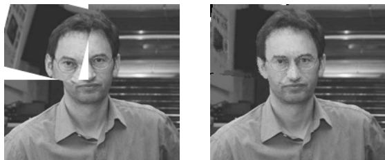
Figura 11b. Block Matching Motion Compensation (rotational motion)
