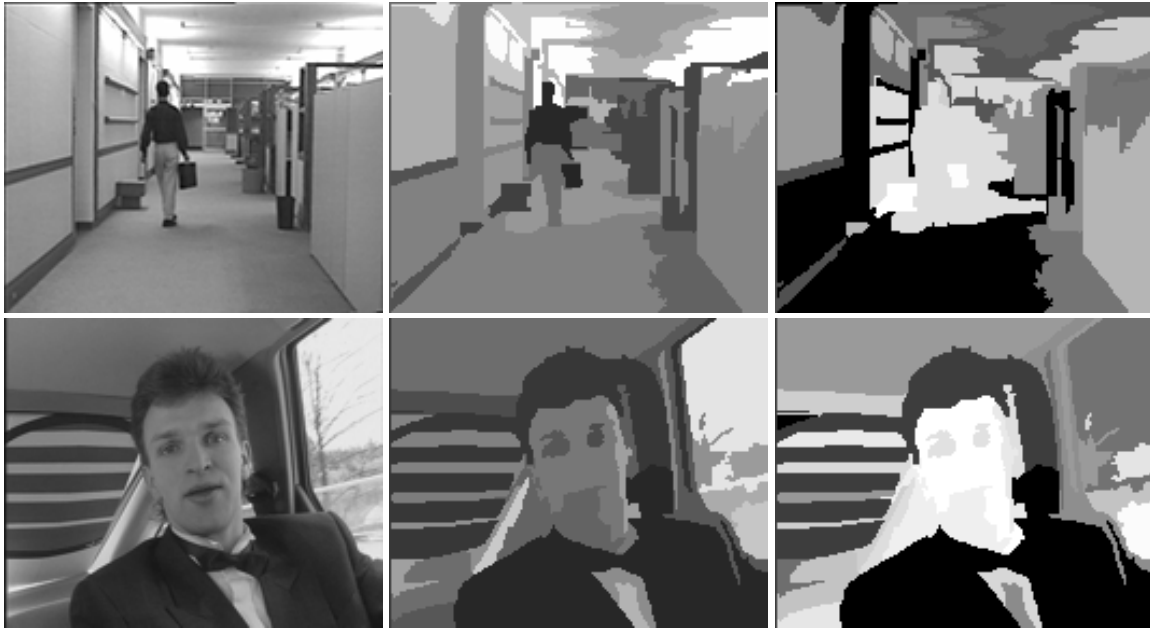
Figure 1: Results for Hall and Carphone images. From left to right: original images, segmented images obtained with our algorithm, and importance map.
