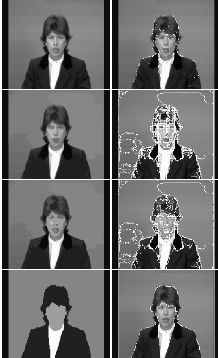
Figure 2: Original Claire image. Detected Tjunctions. Initial segmentation with 1994 regions, after two iterations of VPD (area threshold is 100 pixels) with 766 regions, and the image with six regions matching the semantic objects. In the last three rows we show the image where each region is represented by its mean and the boundaries.
