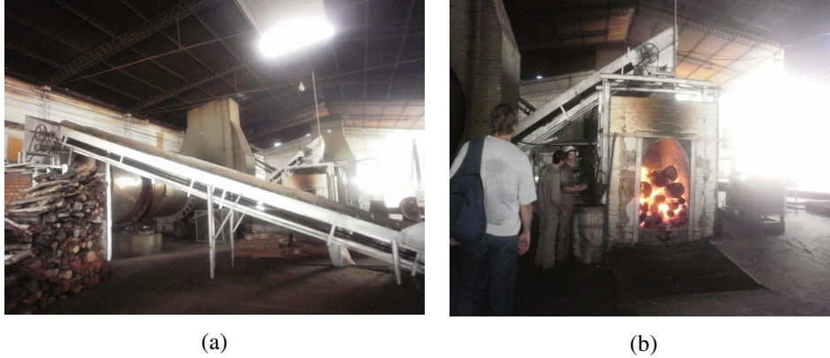
Fig. 1. a) Lateral view of pre-dryer, b) pre-dryer stake.
