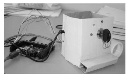
Fig. 2. Key interface developed using phidgets
