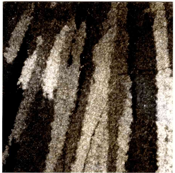
11d Muestra 4. 1180°C - 24hs. Fase: hexagonal 60X
