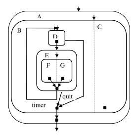
In order to describe and simulate the machine, an Ada task is associated with every state. Each of them includes the declaration of an entry *start* and of a global boolean variable *end\_task*. As an example, the task F of figure 1, associated with a leaf state, is declared and defined as follows:
