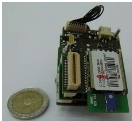
Fig. 2. iSense core and attached modules compared with a coin
