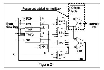
A later elaboration could be to differentiate the access to either RAM or ROM, generating offsets over different memory areas to optimize memory usage. That distinction should be essential when using external RAM/FLASH memories. Besides, this multiple offset scheme can also be used for the definition of shared areas of memory.
