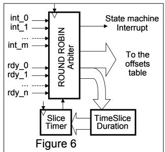
The simplest case is a multitasking system with equal priority tasks, using a "round-robin" arbitration scheme (Figure 6). In this case, the schedule of a new task may have several causes:
