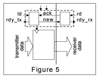
• The other situation is when the receptor is willing to read new data when it is not present (*new* inactive). In that situation the signal *rdy\_rx* remains inactive until the transmitter writes new data.
