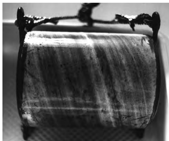
Figure 4. Pipe covered by saturated copper Coating (A) after a month of immersion. Can be observed the loss of copper coating.
