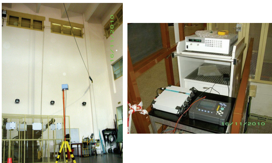
Fig. 4. EFS placed in the High Voltage Lab, under a cable fed with fundamental frequency voltage, harmonics and flicker.
