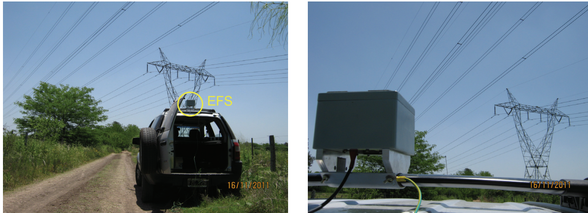
Fig. 5. Electric Field Sensor (EFS) on the roof rack of the vehicle.
