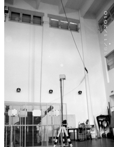
Fig. 3. EFS placed in the High Voltage Lab.
