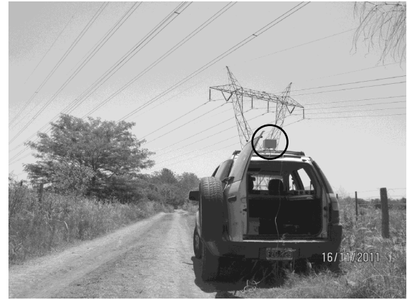
Fig. 4. Electric Field Sensor (EFS) on the roof rack of the vehicle.
