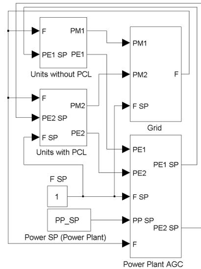
Fig. 7: Power Plant SCL. Simplified block diagram.
