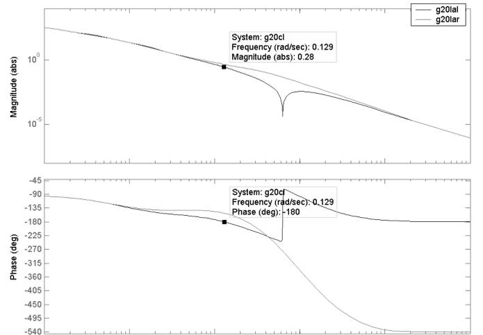
Fig. 12: Open loop Bode diagram. PCL Readjustment 1 (stable)
