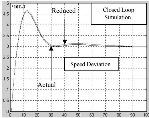
Fig. 5: PCL Model. "Actual" and "Reduced"  $10^{-3} * \Delta\omega$ .
