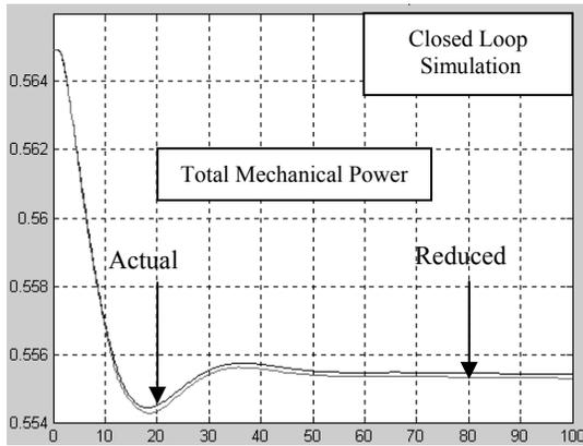
Fig. 6: PCL Model. "Actual" and "Reduced"  $P_M = P_{MT} + P_{MH} + P_{MF}$ .
