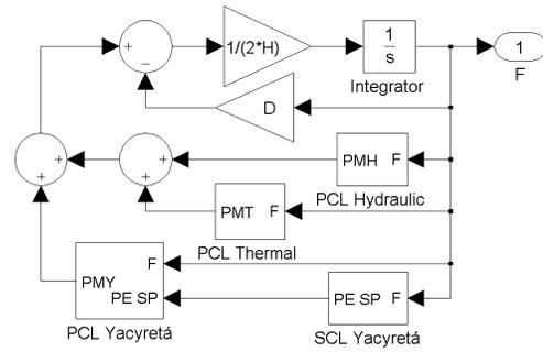
Fig. 10: Complete model for SCL tuning.
