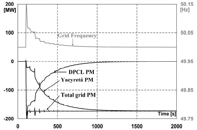
Fig. 18.a. SCL action with Yacyretá PCL Readjustment 2. Mechanical Power in left scale. Frequency in right scale.
