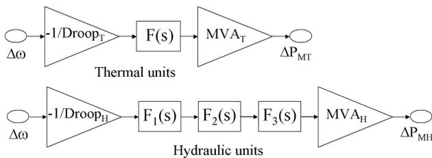
Fig. 2: Equivalent models of thermal and hydraulic units.
