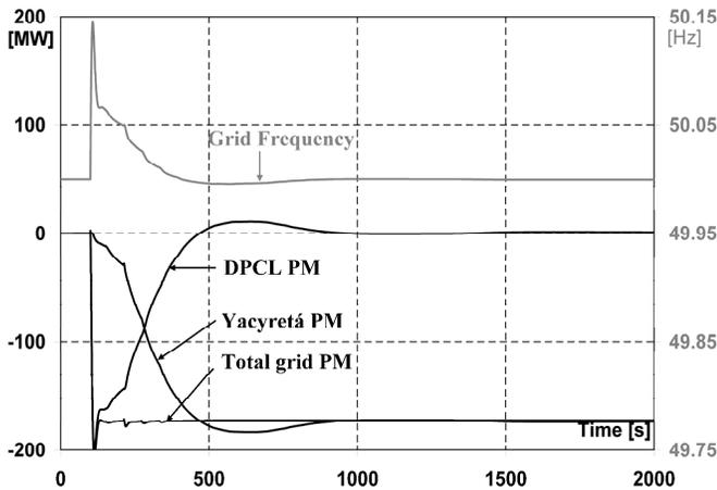
Fig. 17.a. SCL action with Yacyretá PCL Readjustment 1. Mechanical Powers in left scale. Frequency in right scale.
