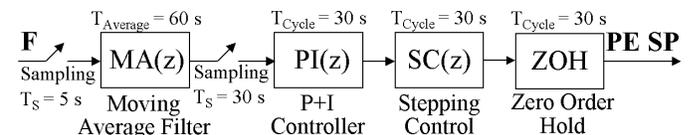
Fig. 8: Simplified block diagram of SCL.
