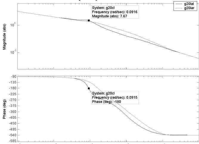
Fig. 11: Open loop Bode diagram. Original PCL (unstable).
