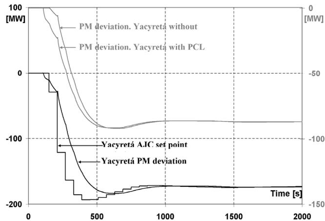
Fig. 17.b. SCL action with Yacyretá PCL Readjustment 1. Lower curves in left scale. Upper curves in right scale.
