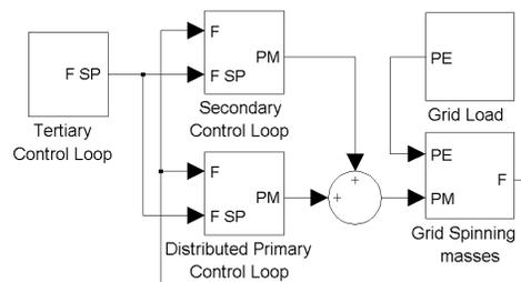
Fig. 1: Grid Frequency Control. Simplified Block Diagram.
