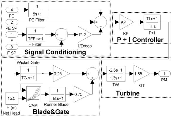
Fig. 9: Linearized model for PCL tuning.
