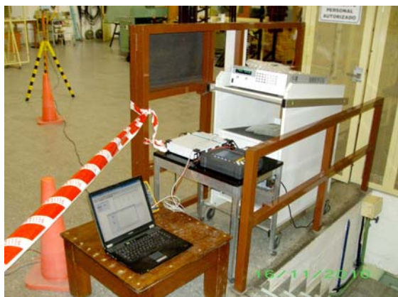
Fig. 3. Electronic power generator, Flicker measured through voltage measurement (black equipment over the table) and Flicker measured through EFS (white equipment).
