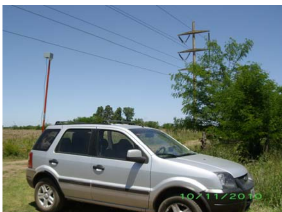
Fig. 6. EFS placement nearby an overhead line.
