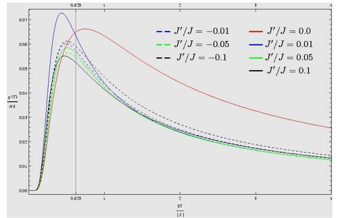
**Figure 3.** Magnetic susceptibility  $\chi(T)$  for a chain of  $N=20$  coupled AF dimers. The red curve ( $J'/J = 0$ ) corresponds to an isolated AF with  $J = -400\text{K}$ . The vertical line at  $kT/|J| = 0.625$  indicates the maximum of  $\chi(T)$  calculated with the Bleaney-Bowers' equation (5).
