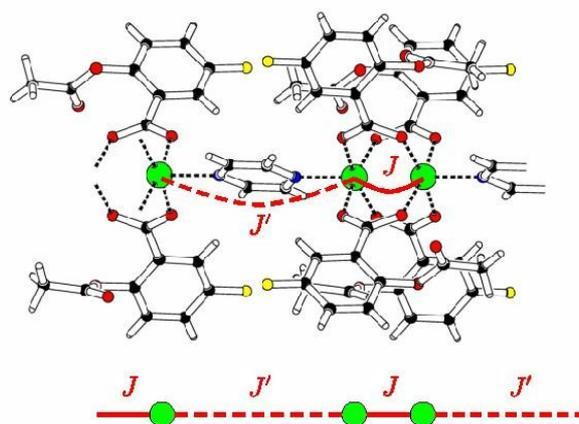
**Figure 2.** Molecular diagram showing part of the  $[\text{Cu}(\text{Fasp})_4\text{Cu}(\text{pyz})]_n$  polymer and the labeling of the super-exchange coupling constants referred to in the theoretical calculations. Large green disks indicate Cu(II) ions, while the red, blue, yellow and black smaller disks denote oxygen, nitrogen, fluorine and carbon atoms, respectively.
