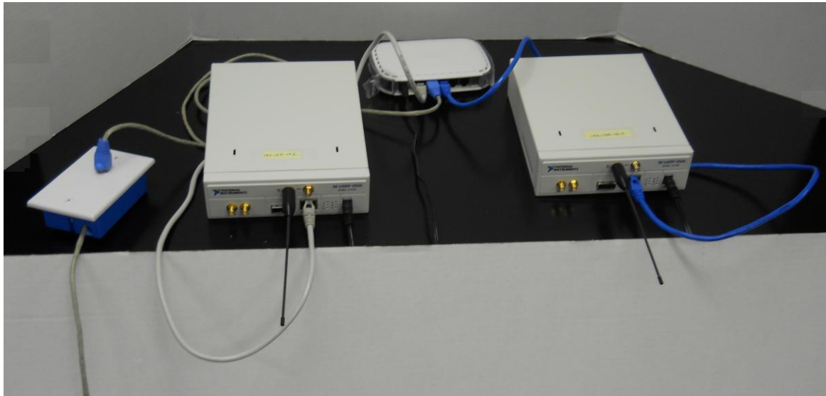
Fig. 7: P2PW Wireless Setup
