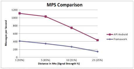
**Fig. 2.** QoS *calculateMPS* vs Android API bandwith funcion, depending on Signal Strength. Values are normalized to *Messages Per Second* for a correct visual interpretation.
