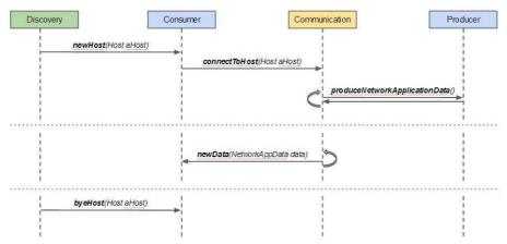
**Fig. 4.** Sequence and interaction diagram. *Discovery* and *Communication* are components of the framework. *Consumer* and *Producer* are application-level subclasses of *NetworkApplicationDataConsumer* and *NetworkApplicationDataProducer*.
