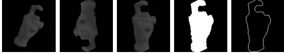
Figure 3: From left to right: Segmented image, oriented image, image with corrected rotation, hand segmentation mask, and contour.
