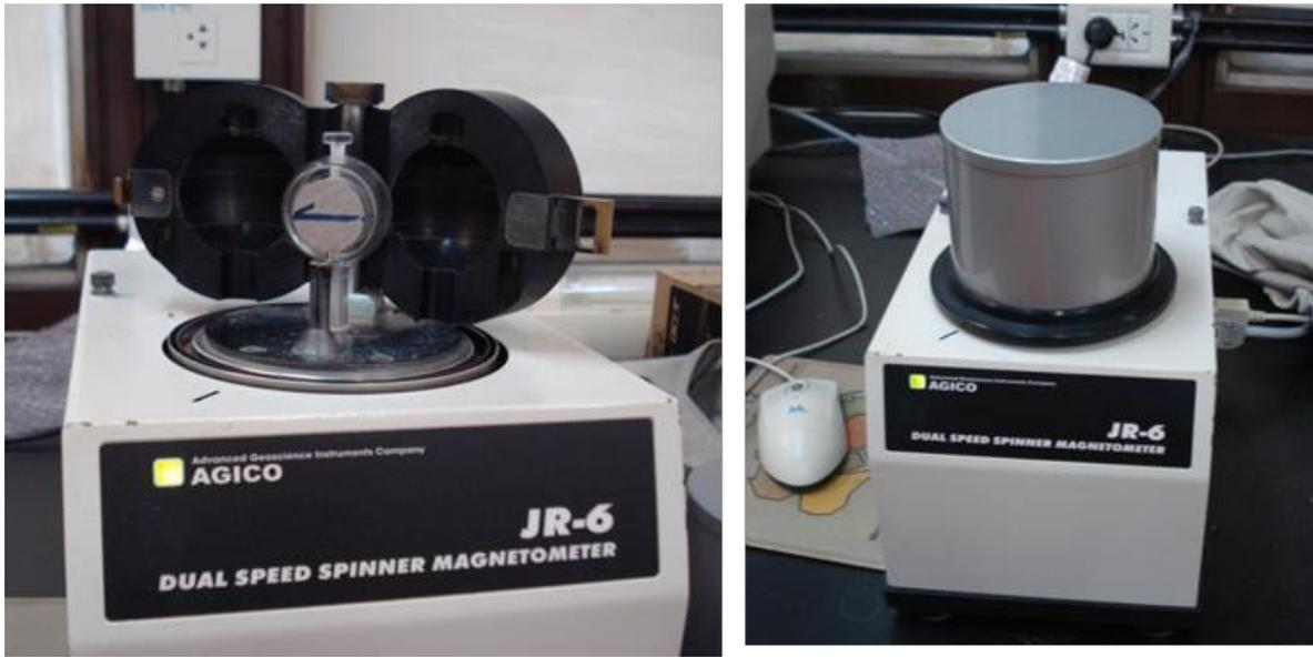
Figura 4.9. Magnetómetro JR-6 AGICO Dual Speed Spinner magnetometer.
