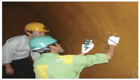
Open-tank wall thickness measurement The thickness of the tank wall is measured from inside the tank for safety verification.
