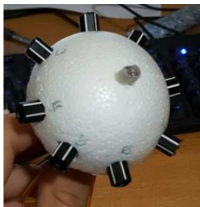
Figure 3: The semi-sphere shape sensor showing the position of the LDRs.
