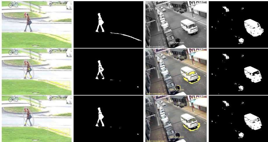
Fig. 4. Background subtraction and shadow detection. Original image or Object contour with detected shadow (left) and resulting mask (right). ViBE algorithm (top). Shadow detection algorithm with NCC (center) and Shadow detection with the proposed algorithm (below)
