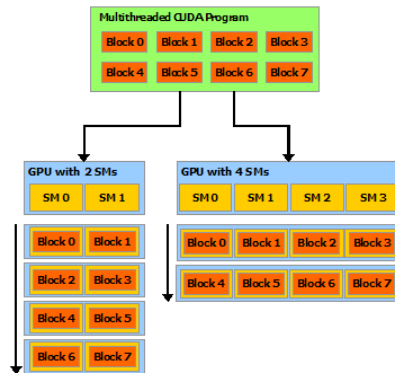
Fig. 1. From [6]: A multithreaded program is partitioned into blocks of threads that execute independently from each other, so that a GPU with more multiprocessors will automatically execute the program in less time than a GPU with fewer multiprocessors. To solve the problem. In this way scalability is easily achieved, see Figure 1. To understand image filtering implementations on GPUs, and to make this article self-contained, we first review the basics using a simple examples of vectors and matrices addition (This section is based on [6]).
