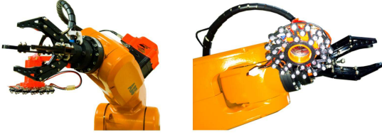
Figure 5: Left, robot gripper and camera. Right, LED support mounted around the camera.
