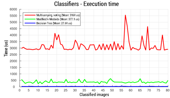
Figure 12: Algorithm execution time comparison.
