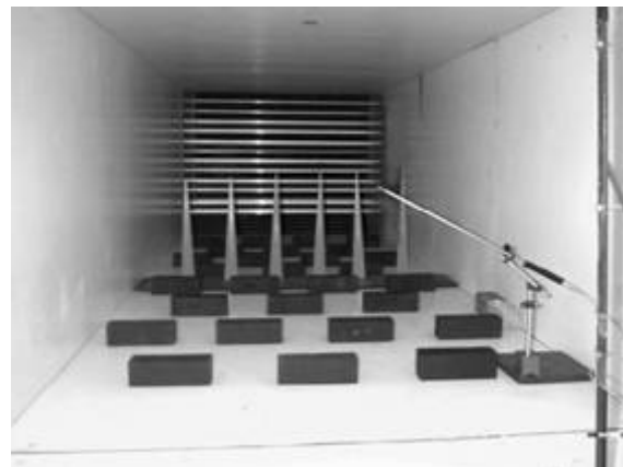
Fig. 3 – Wind Tunnel layout for turbulence characterization
