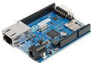
**Figura 2:** Arduino ethernet shield.
