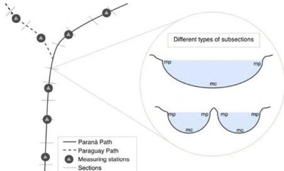
Fig. 1 Discretization of the simulated domain river system.
