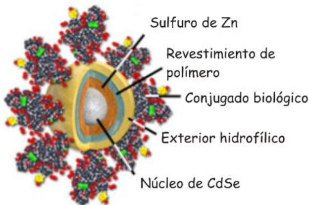
**Fig. 3-28.** Nanocristal fluorescente (Quantum dot - Qdot).
