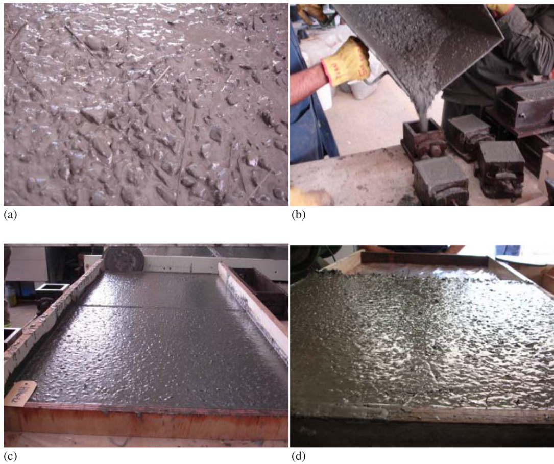
Fig. 1. Specimens preparation: (a) Concrete aspect (b) Filling of concrete cubes (c) HSC slab and (d) HSFRCC slab.
