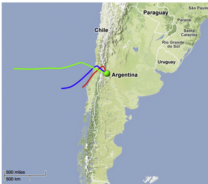
Fig. 6. Example of a back trajectory from the Malargüe location using HYSPLIT. The initial height is fixed at 500 m above ground level for the red line, 1000 m for the blue line and 3000 m for the green line (map taken from Google Earth).
