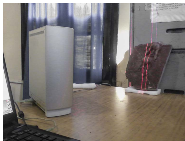
Figure 6. Manus-pes set F2 from Trackway 2 (see Krapovickas and Nasif, 2011) being scanned at the police station.
