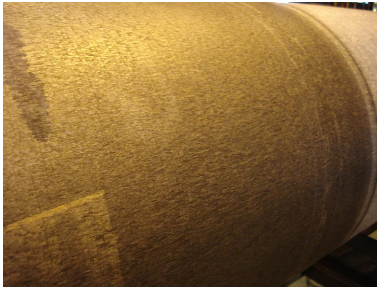
Figura 2. Vista del rodillo conductor atacado Figure 2. Corroded conductor roll
