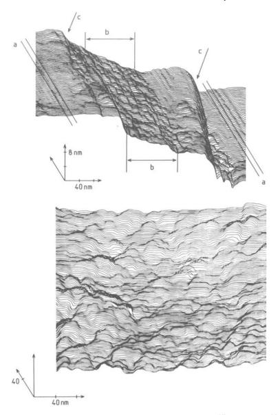
Fig. 10. (a) STM imaging of a Pt surface with a roughness factor of 80. Three different topographies can be distinguished (a, b, c). Regions of type b are responsible for high values of the roughness factor: (b) STM imaging of Au surface with a roughness factor of ≈ 80.
