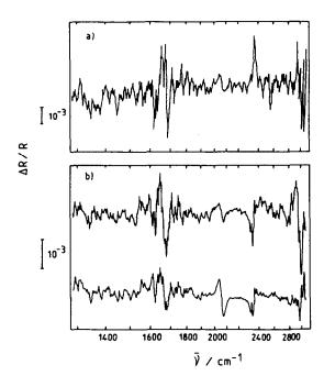
Fig. 7. EMIRS spectra of the species resulting from methanol adsorption on pc Pt as a function of the number of scans, ie of the adsorption time; 0.5 M HClO<sub>4</sub> +  $5 \times 10^{-3}$  M CH<sub>3</sub>OH,  $\Delta E = 0.4$  V,  $\bar{E} = 0.2$  V/rhe, f = 13.5 Hz, room temperature: (a) first scan; (b)  $10^{th}$  and  $25^{th}$  scans.
