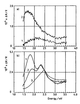
Fig. 11. (a) Electroreflectance spectra of smooth (1) and electrodispersed platinum (2); 0.3 M HClO<sub>4</sub>;  $\bar{E}=-0.25$  V vs mse;  $\varphi=40^\circ$ , p-polarization; f=22 Hz;  $\delta E=30$  mV<sub>(rms)</sub>; (b) Electroreflectance spectra of electrodispersed Au (1, 2) and pc smooth Au (3); 0.3 M HClO<sub>4</sub>;  $\bar{E}=0.1$  V vs mse (1) and  $\bar{E}=-0.3$  V vs mse (2, 3);  $\varphi=40^\circ$ ; p-polarization; f=180 Hz;  $\delta E=28$  mV<sub>(rms)</sub>.
