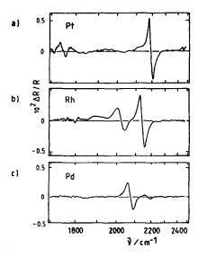
Fig. 5. EMIRS spectra of CO species adsorbed on noble metal electrodes immersed in a 0.5 M HClO<sub>4</sub> solution saturated with gaseous CO.  $\Delta E = 400$  mV,  $\bar{E} = 0.2$  V vs rhe, f = 13.5 Hz: (a) Pt; (b) Rh; (c) Pd.
