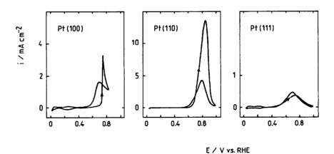
Fig. 9. Voltammograms of Pt(100), Pt(110) and Pt(111) single crystal electrodes in 0.5 M HClO<sub>4</sub>+0.1 M CH<sub>3</sub>OH solutions at 25°C and v=50 mV s<sup>-1</sup>; only the first sweep is represented.
