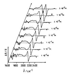
Fig. 14. Series of EMIRS spectra of the adsorbed layer formed at a upd modified Rh electrode in 0.1 M HCOOH +0.25 M HClO<sub>4</sub> + x M Pb<sup>2+</sup> solutions (x was varied from  $5 \times 10^{-7}$  M to  $1 \times 10^{-3}$  M, as indicated in the figure). Spectral conditions:  $\Delta E = 0.4$  V; E = 0.2 V vs rhe, f = 13.5 Hz; 10 averaged scans.
