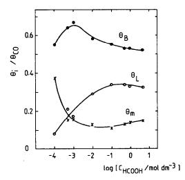
Fig. 13. Dependence of the relative coverage by each type of adsorbed CO species at a Rh electrode on the concentration of HCOOH in 0.25 M HClO<sub>4</sub>:  $\Theta_L$ ,  $\Theta_B$  and  $\Theta_m$  correspond to linearly bonded CO, two-fold and multi-fold bridge-bonded CO, respectively.
