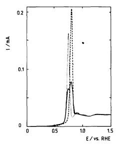
Fig. 4. Voltammograms of adsorbed CO electrooxidation on polycrystalline(——), type I (...) and type II (---) platinum electrodes. Adsorption potential  $E_{\rm ad} = 0.25 \, \text{V/rhe}$ ; adsorption time  $t_{\rm ad} = 1 \, \text{min.}$ , sweep rate,  $v = 0.1 \, \text{V s}^{-1}$ ; 0.05 M HClO<sub>4</sub>; 25°C. For the preparation of type I and type II electrodes[18].
