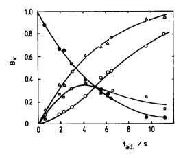
Fig. 2. Adsorption of CO on a pc. Pt electrode immersed in a 1 M HClO<sub>4</sub> solution saturated with gaseous CO. The degree of surface coverage,  $\Theta$ , by the two adsorbed species, CO<sub>L</sub> and CO<sub>B</sub>, is given as a function of  $t_{ad}$ .  $E_{ad} = 0.59 \text{ V/rhe}$ , 25°C:
