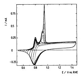
Fig. 1. Voltammograms of a polycrystalline Pt electrode in a 1 M HClO<sub>4</sub> solution saturated with gaseous CO, at different lower potential limits,  $E_c$  ( $v = 100 \text{ mV s}^{-1}$ ; 25°C): (°°°) = 0.80; (·°·°) = 0.71; (-xx-xx-) = 0.74; (-·····) = 0.71; (-x-x-) = 0.65; (·····) = 0.62; (····) = 0.59; (····) = 0.56; (·····) = 0.53 V.
