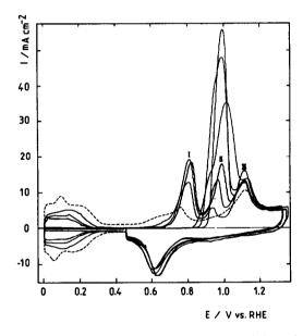
Fig. 3. Voltammograms of a Pt(111) single crystal electrode in 0.5 M HClO<sub>4</sub> saturated with gaseous CO for different adsorption times  $(1.2 < t_{ads} < 25 \text{ s})$ .  $E_{ads} = 0.45 \text{ V/rhe}$ ; 25°C;  $v = 10 \text{ V s}_{-1}^{-1}$ ; (---) = supporting electrolyte.
