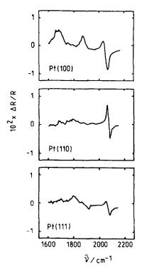
Fig. 8. EMIRS spectra of the adsorbed CO species resulting from the chemisorption of 0.1 M CH<sub>3</sub>OH in 0.5 M HClO<sub>4</sub> at a Pt single crystal electrode;  $\Delta E = 400 \text{ mV}$ ,  $\bar{E} = 350 \text{ mV/rhe}$ , f = 13.6 Hz, exposed face: (a) Pt(100); (b) Pt(110); (c) Pt(111).
