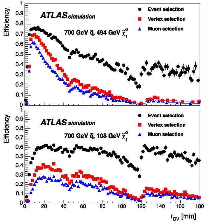
**Fig. 3.** The efficiency as a function of  $r_{DV}$  for vertices in the signal MC samples MH (top) and ML (bottom) of Table 1. In each plot, the top histogram (circles) is the efficiency for the event selection criteria, the middle histogram (squares) shows the efficiency when also requiring one vertex to satisfy the vertex-selection criteria, and the bottom histogram (triangles) includes the muon-selection criteria. The material veto is not applied when making these plots.
