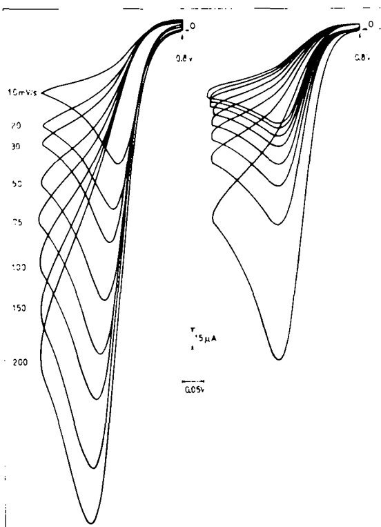
Fig. 10. Voltammograms run in the cathodic direction. 5.30 \times 10^{-2} M HCl, 1.20 \times 10^{-3} M HAuCl 4 , 1 M NaClO 4 , 26.2^\circ C . (a) Effect of v_s ; (b) repetitive triangular potential scans at 75 mV s^{-1} .
