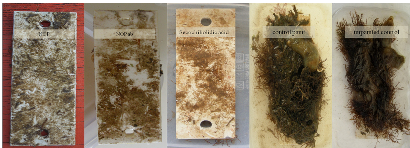
Fig. 3. Painted panels after immersion time.
