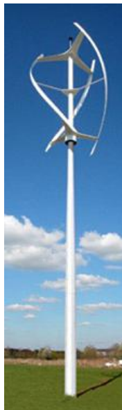
Fig. 2.5: Turbina Darrieus(EcoSources [Blog Internet], 2008)
