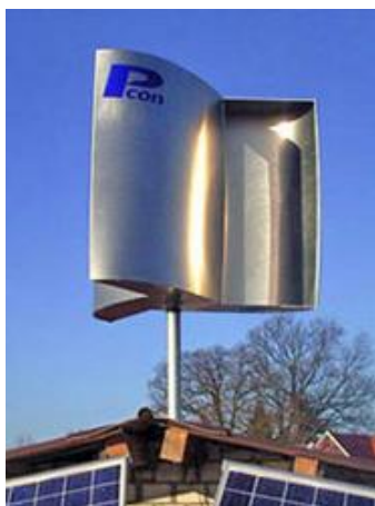
Fig. 2.4: Turbina Savonius(EcoSources [Blog Internet], 2008) Ecosources.info. (2008)
