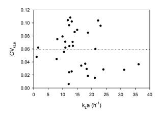
**Figure 2:** Coefficient of variation of  $k_{La}$  ( $CV_{kLa}$ ) as a function of the  $k_{La}$  value in a 500-mL respirometer. All measurements are triplicates at least. The dotted line indicates the overall mean value of  $CV_{kLa}$ .
