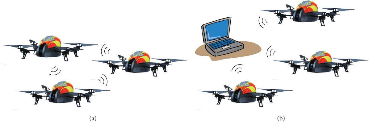
FIGURE 1: Network topology of the different architectures implemented in quadrotors. (a) Local distributed topology. (b) Supervised global topology.
