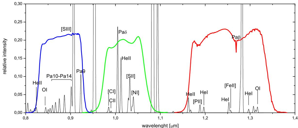
**Fig. 1.** Transmission curves for the Z, Y and J broad-band filters (the effective wavelengths are 0.878, 1.021 and 1.254  $\mu\text{m}$  respectively), the filters are multiplied by a model atmosphere. The spectrum of the PN IC 5117 is superimposed (Rudy et al. 2001), scaled to  $\text{Pa}\beta = 1$ .
