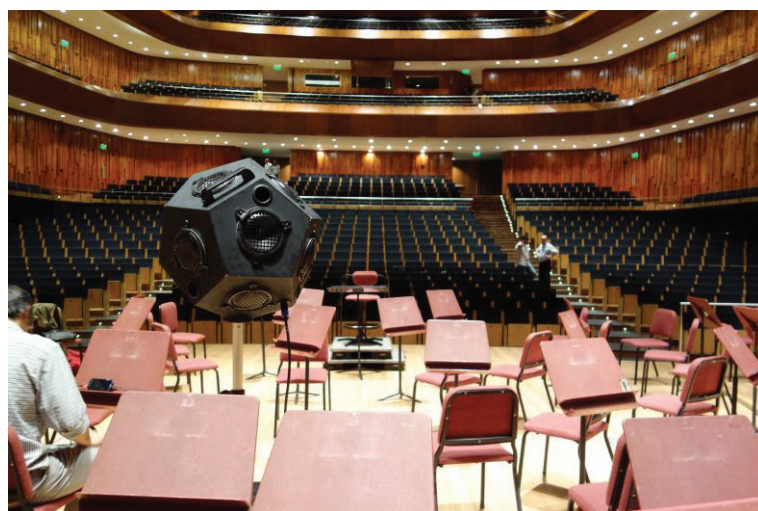
Figure 8: Dodecahedral speaker used in the 2016 measurements (IADA E)
