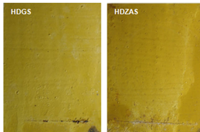
Fig. 4. Photograph of the samples after 150 days of exposure in HC.
