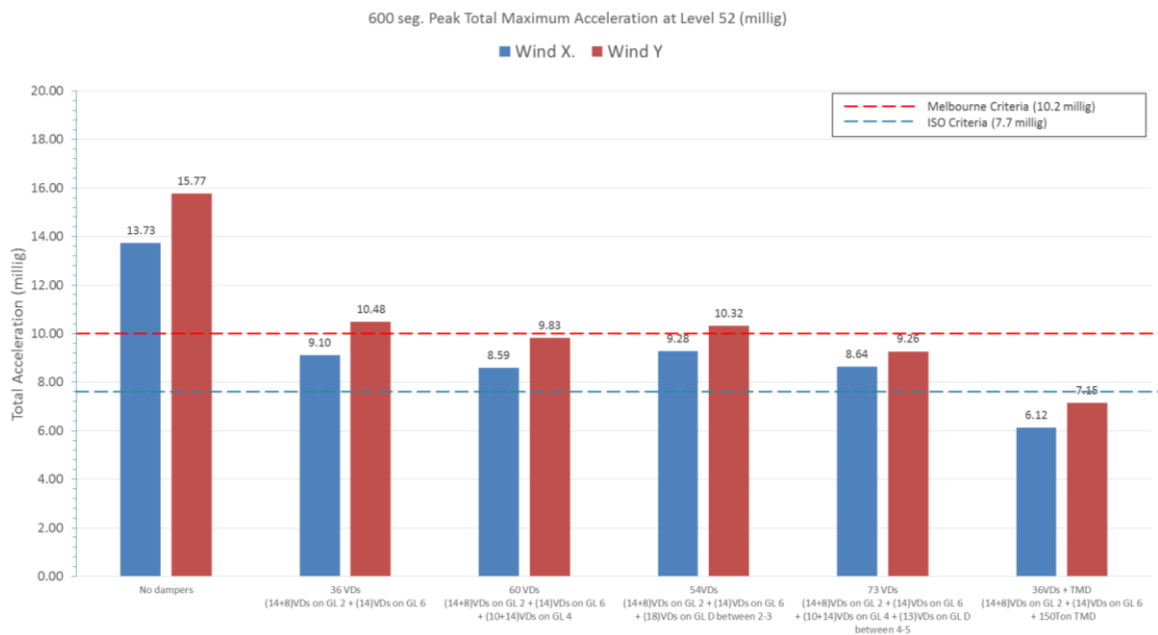
Figure 13. Summary of maximum peak accelerations at Level 52 obtained for damper configurations
