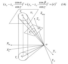
Fig.4. Perspective projection of circular feature So the rays coming from the circle  $\Gamma_1$  located on the plane  $\Pi_1$  form a skewed cone, whose boundary curve can be expressed as:
