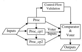
Figure 1. Schematic Diagram of a Single-Version Scheme (SVS).
