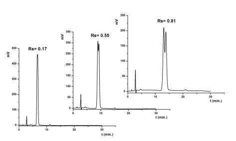
**Figure 2.** Superimposed chromatograms of partially overlapped profiles of *S:R* 95:5 ketoprofen. Chromatographic conditions as in Figure 1. Eluent compositions: see Table 3.
